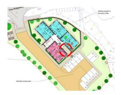
I am a little concened about the significant recess in proximality to the door. It is always recommended that recesses are less than 600mm so they do not provide areas to hide. Obviously I do aprpeciate that there may be limitations with the design of the door etc. If the recessed are is to stay consideration should be given to appropriate lighting and CCTV coverage.
